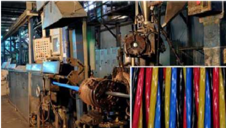
Extruding Machine for Insulation
