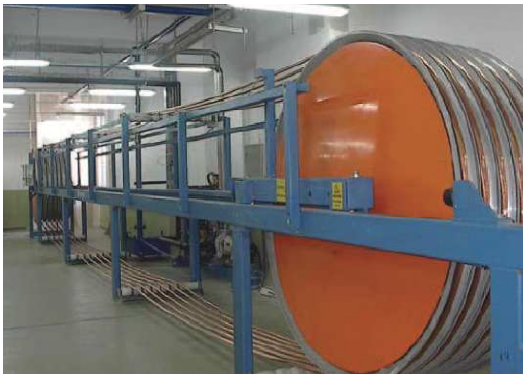
Accumulator in the CV-Line
